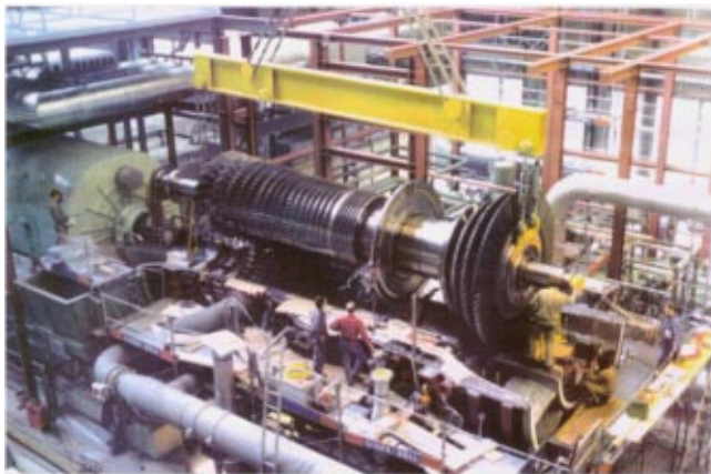
Fig. 18 GT 26 rotor assembly at the ALSTOM Power GT Test Center, Birr, Switzerland
