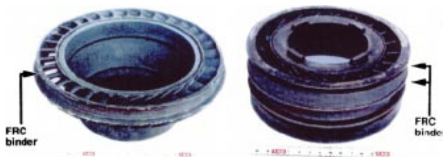
Fig. 5 FRC bound GGT and PT nozzles
