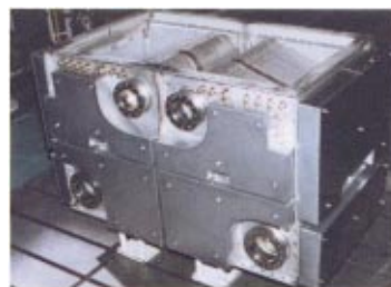
Fig. 18 Recuperator of CGT302 (49+49 fins for each core)
