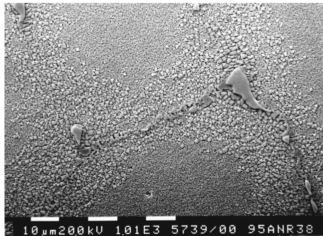
Fig. 8 A scanning electron micrograph of an IN-738LC turbine blade not correctly processed through the modified high-temperature reheat treatment cycle
