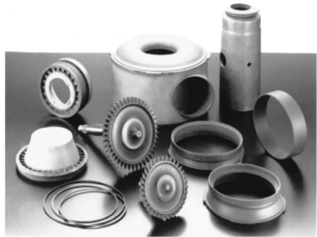
Fig. 2 All the ceramic parts of CGT302
