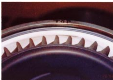
Fig. 6 Abradable PT shroud after engine test
